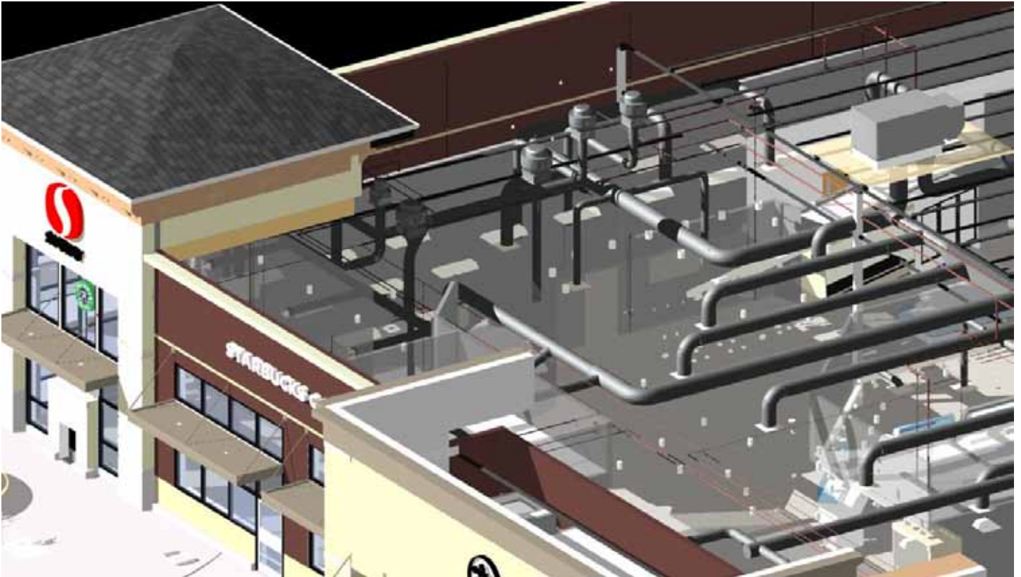
(Above) A data-rich BIM model, that can be plugged into other MEP projects, provides comparative information about cost, scheduling, and equipment options. Any change to the model ripples through and updates the outcomes, reducing data entry errors and document coordination mistakes. (Below) One of Safeway's first locations, in Medford, Oregon, developed using a BIM model. (Right) The Longview, Washington store was also designed according to the BIM prototype.
